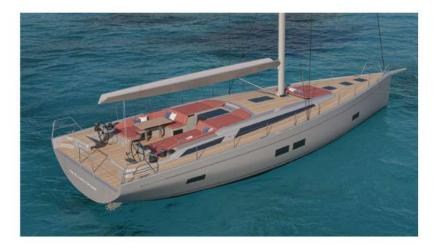
The GS 60 LC is tailored to deliver classic LC features, prioritizing exceptional comfort and easy sailing while maintaining optimal performance. Noteworthy design elements include a pronounced V-shaped bow, low-wet surface, and outstanding dynamic stability.
